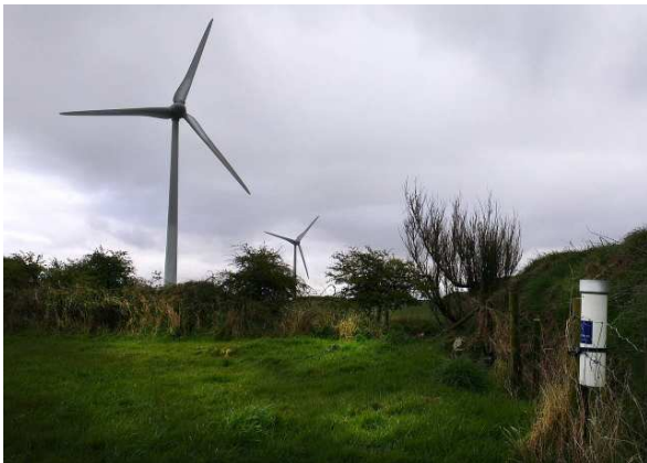
Figure 1: Pluviometer deployed in a field adjoining a wind farm (photo by courtesy of Hayes McKenzie Partnership Ltd)
