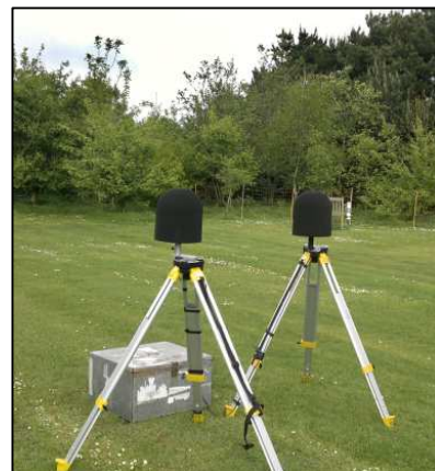
Figure 2: Noise monitoring equipment deployed for measurement of sound levels generated by wind turbines (photo by courtesy of Hayes McKenzie Partnership Ltd)
